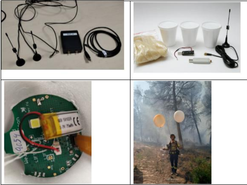
Figure S1.- The measurement kit detail. a) data logger with the reception antennas. b) reusable sondes in Styrofoam cups and latex balloons. c). Detail of the sonde sensors with battery inside the Styrofoam cups. d).- Balloons and sondes attached ready to be used. On average, the system is ready in as little as 8 minutes, allowing smooth and safe operations at the fire.
