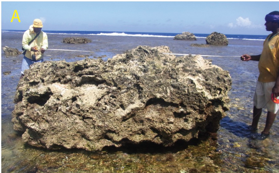
Fig. 4. Some field method techniques. A.: tape measurement of boulder axes; the irregularity of this boulder means that volume or mass estimates from tape dimensions are approximation only. B: Siting a photogrammetric ground control point using RTK GPS. C: Site surveying for elevation measurements using a transit compass (Brunton), which in combination with tape or laser rangefinder distance measurements can be used to derive vertical and/or horizontal distance using trigonometry. D: measuring boulder distance from a shoreline marker using a laser rangefinder.. (Photo A by Annie Lau, B-D by Rónadh Cox,)
