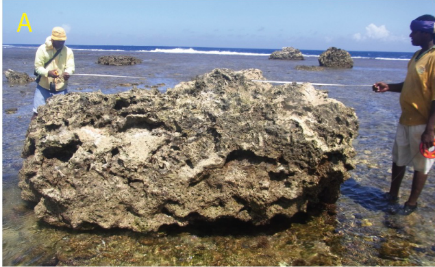
Fig. 4. Some field method techniques. A.: tape measurement of boulder axes; the irregularity of this boulder means that volume or mass estimates from tape dimensions are approximation only. B: Siting a photogrammetric ground control point using RTK GPS. C: Site surveying for elevation measurements using a transit compass (Brunton), which in combination with tape or laser rangefinder distance measurements can be used to derive vertical and/or horizontal distance using trigonometry. D: measuring boulder distance from a shoreline marker using a laser rangefinder.. (Photo A by Annie Lau, B-D by Rónadh Cox.)
