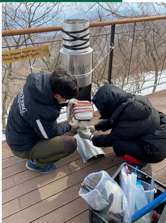
Figure R1-1. Installation and sampling procedure of the rainwater collector at the ski resort site. The photo shows researchers collecting precipitation using a stainless-steel rain sampler designed to prevent contamination and minimize evaporation losses.
