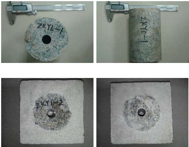
Figure 2: Photo of hydraulic fracturing cuboidal specimen
