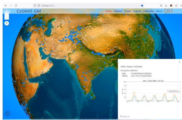
Figure 888: Django Web User Interface for visualising and managing the CoSWAT Global Model ( https://github.com/celray/coswat )
