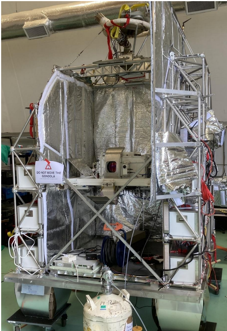
Figure 2. GLORIA-B instrument after integration into the balloon gondola.
