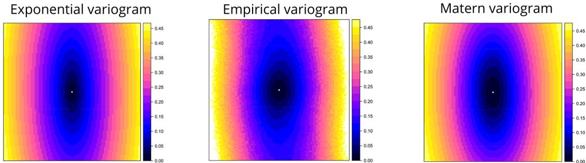
Here are the empirical variogram and the fitted exponential and Matérn variograms for a given day. The exponential variogram fits the empirical one well, benefiting from the large number of estimation pixels used as virtual gauges. However, the Matérn variogram appears to better capture the short-range spatial variability, providing a smoother representation than the exponential variogram. A cross-validation would be needed to assess the best variogram for precipitation interpolation.
