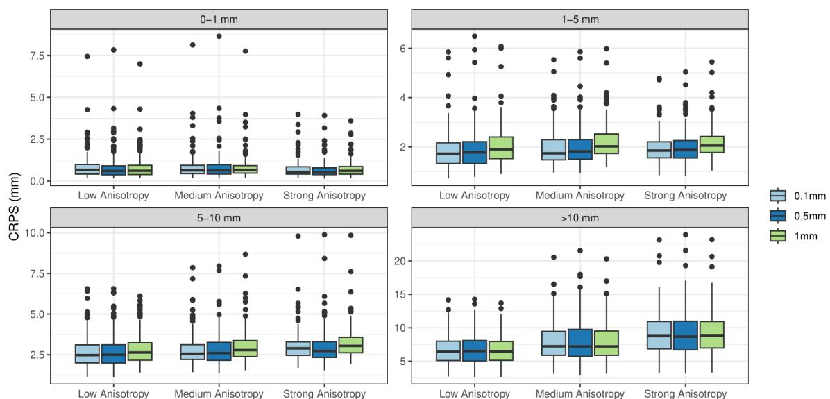
The above figure highlights the CRPS score with the arANISO model. A too high threshold (1 mm) leads to bias for moderate precipitation (1-5 mm, 5-10 mm), and a too low threshold (0.1 mm) degrades the estimation of 0-1 mm. 0.5 mm corresponds to a good compromise.
