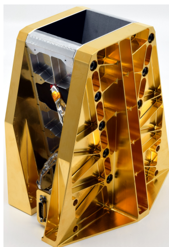
Figure 3. The Arctic Weather Satellite onboard calibration target.
