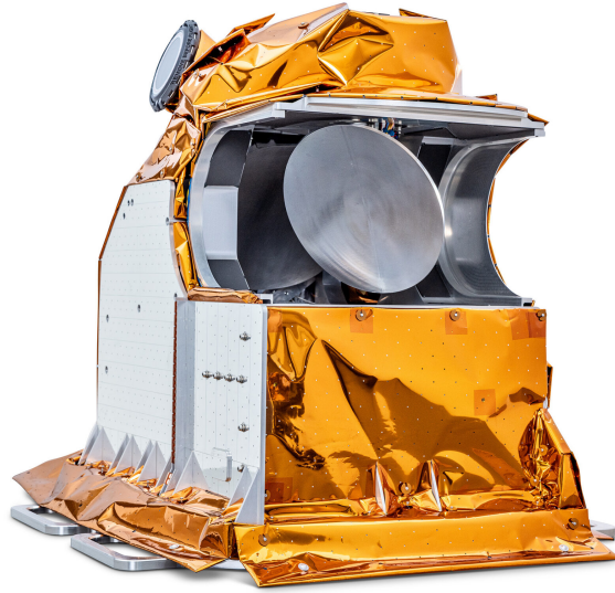
Figure 1. Photo of the Arctic Weather Satellite payload, a 19-channel microwave cross-track sounder. The metallic plates on the left side are thermal radiators. Above these, one of the two star trackers can be discerned. The scanning is achieved by the elliptical mirror, in the photo seen pointing to the left. The mirror is attached to an axis above it and directing radiation to the radiometer package below it. The front side will in space be facing the nadir direction.
