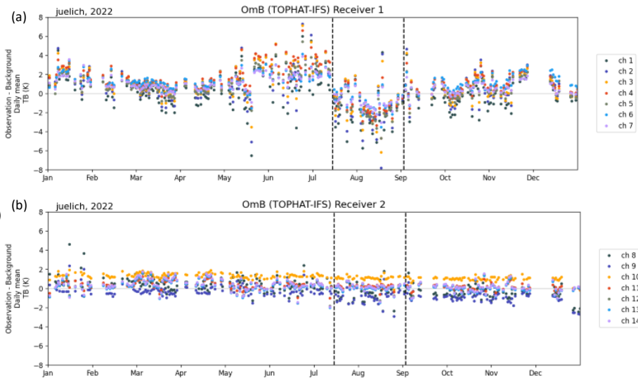
Figure 55: Daily means of OmB brightness temperature differences for TOPHAT at JOYCE during 2022, (a) for K-band (Receiver 1) and (b) V-band (Receiver 2). The dashed lines indicate times of LN2 calibrations. Observations and background are clear-sky only.
