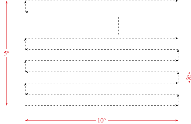
Figure 5. Illustration of the box scan that is performed around the virtual target.
