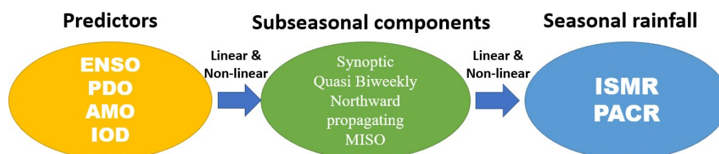
Figure 6. A schematic diagram illustrates how slowly varying predictors influence seasonal rainfall anomaly by modulating sub-seasonal components. The sub-seasonal components are considered the building blocks of seasonal rainfall.
