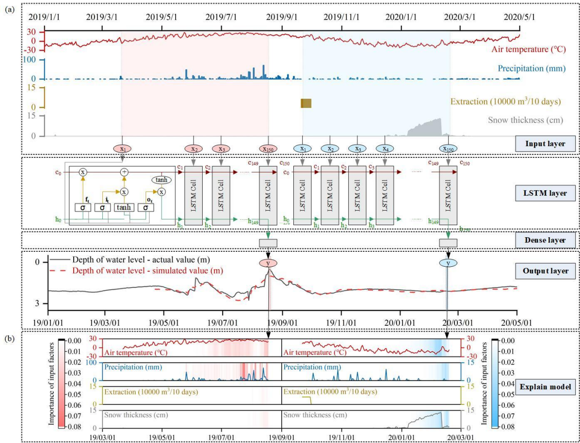
Fig. 1. Workflow of this study: (a) Model structure of the LSTM model, (b) EG scores of input factors during the non-freeze-thaw and freeze-thaw periods.
