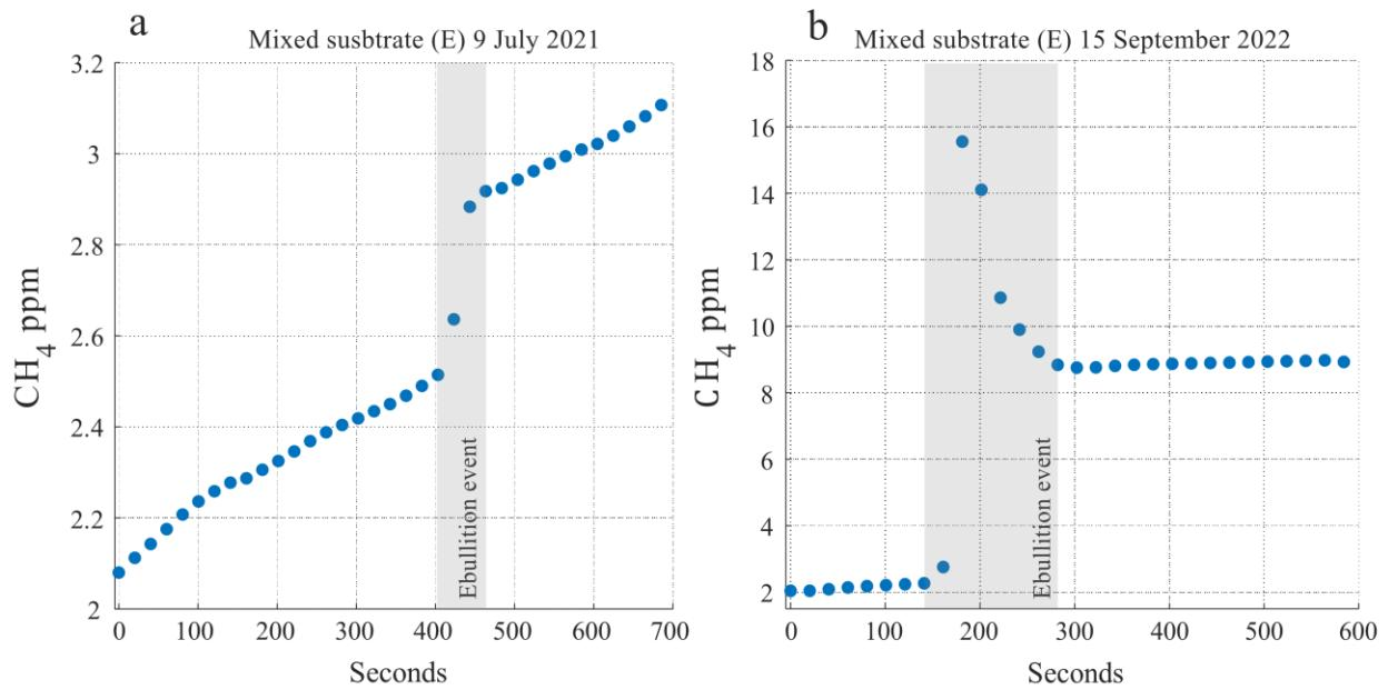
**Figure S1.** Raw data from the GGA showing two (A and B) ebullition events, both captured in sampling location E. The blue dots indicate how the concentration of  $\text{CH}_4$  in the chamber system changes as a function of seconds elapsed since the start of the incubation. The abrupt changes marked in grey are interpreted as ebullition events and indicate the start and end time of the ebullition used for calculating the flux.
