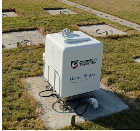
Figure 1. Installation diagram of the wind lidar.
