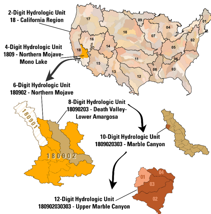
Figure 1: Watershed Boundary Dataset structure. From: US Geological Survey. Watershed Boundary Dataset. 20250204 https://www.usgs.gov/national-hydrography/watershed-boundary-dataset . Public domain.
