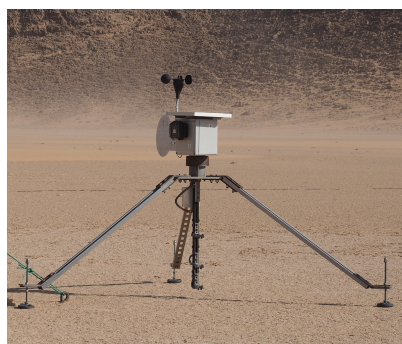
Figure 3. SANTRI instrument to measure saltation and retrieve flux density to obtain threshold friction velocity.
