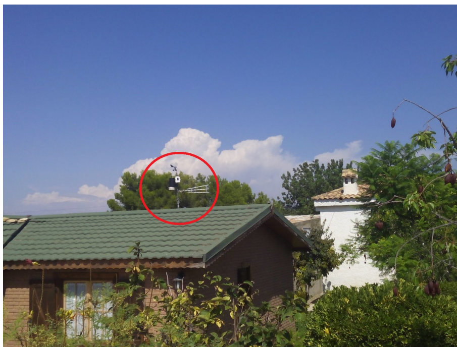
Figure C1. Installation setup from the Davis PWS in Túrís that recorded over 600 mm on 29 October 2024, obtained from: https://www.avamet.org/mx-fitxa.php?id=c20m248e02 , last access: 28 November 2024. The PWS is indicated by the red circle.
