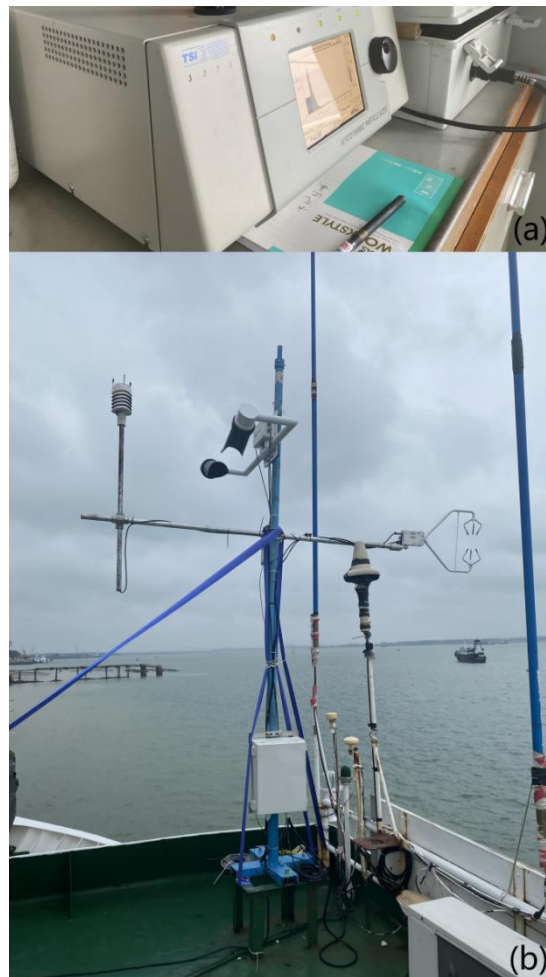
210 | Fig. 21 The total view of (a) the Model 3321 APS spectrometer and (b) the automatic meteorological observation system.
