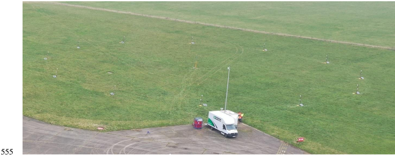
Figure A1. Aerial photograph of the validation setup (see also Fig. 2). The FEDS trailer can be seen in the centre foreground of the image (behind the van) with the 10 m meteorological mast attached to the trailer. The 12 sampling locations are arrayed in a circle on the grass beyond the trailer with the CRF release location in the centre.
