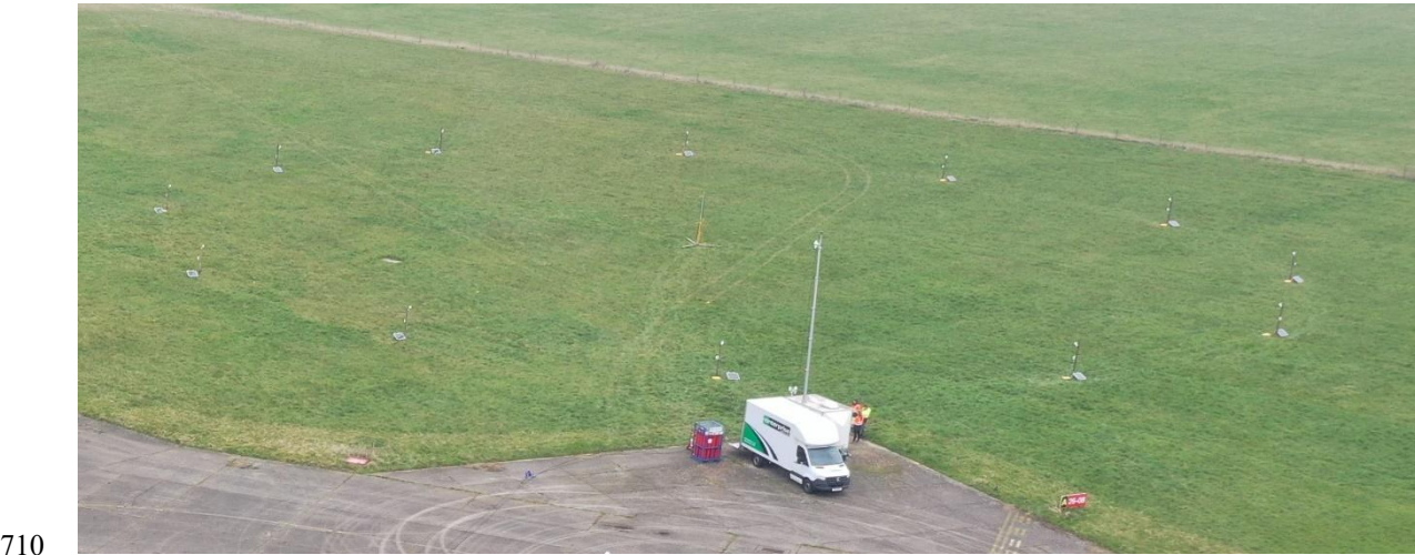
710 Figure A1. Aerial photograph of the validation-field setup (see also Fig. 2). The FEDS trailer can be seen in the centre foreground of the image (behind the van) with the 10 m meteorological mast attached to the trailer. The 12 sampling locations are arrayed in a circle on the grass beyond the trailer with the CRF release location in the centre.
