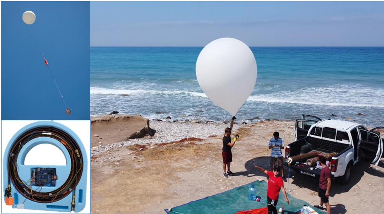
Figure S2: Photos from Nicosia, Cyprus AirCore campaign. A cross section of our AC sampling system (lower left) and the AC just launched (upper left). Here, we use a low-resolution AC device from LSCE built as a double stainless-steel, coated tubing of 35 m long, consisting of a 12 m long 8 mm in diameter tube and a 23 m long 4 mm in diameter tube. The vertical air samples were analysed with a cavity ring-down spectrometry (CRDS) gas analyzer by Picarro, model G2401. Right: photo from the AC launch of 30 June 2020.
