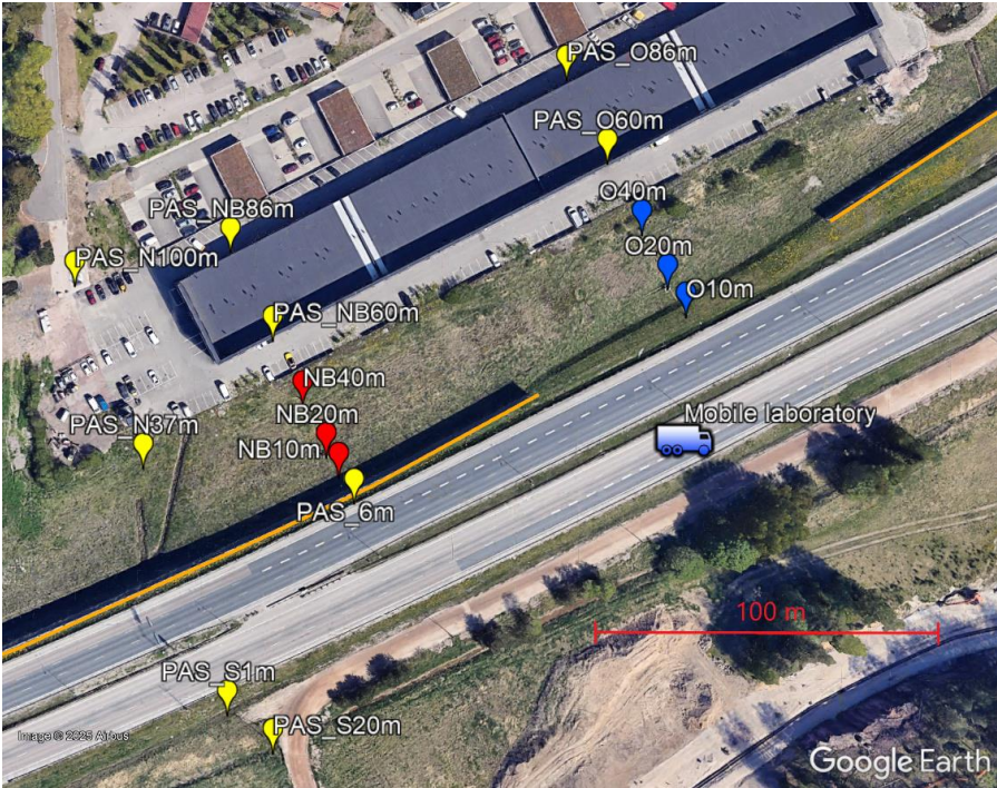
Figure 1: Measurement infrastructure at the measurement site. The noise barrier has been marked to figure with orange lines. The measurement poles behind the noise barrier (NB10m, NB20m, and NB40m) have been marked with red, and the measurement poles in the open area (O10m, O20m, and O40m) have been marked with blue. Passive NO 2 samplers (PAS_N100m, PAS_N37m, PAS_S1m, PAS_S20m, PAS_6m, PAS_NB60m, PAS_NB86m, PAS_O60m and PAS_O86m) have been marked in yellow. There were also passive samplers located in the main measurement poles. Also, a mobile laboratory is presented in the figure. (© Google Earth 2024)
