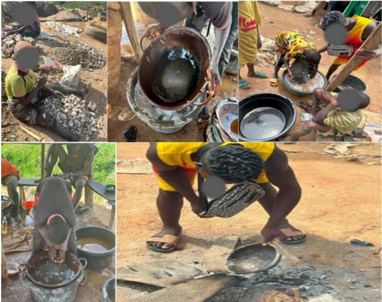
Figure S1.2: Processing of gold ore at the ASGM Processing Site (PS) in Uke. Activities involve crushing and grinding ore, addition of Hg for amalgamation, and burning off the amalgam.
