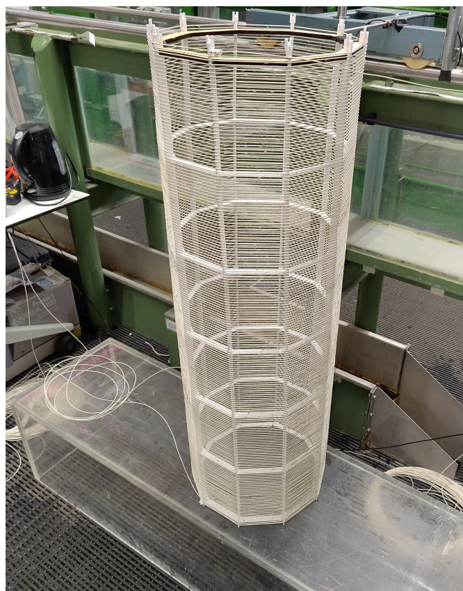
Figure 1. Top view of the final coil geometry. Here the structure of the frame is clearly visible. Vertical support ribs are slotted into a series of rings, which form a rigid frame using a minimal amount of material. The DTS fiber optic cable is wound around the frame and spirals helically upward to its top.
