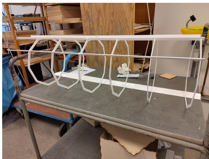
Figure 4. The parts of the frame being assembled. Ribs are slotted into the array of support rings one by one to construct the frame.
