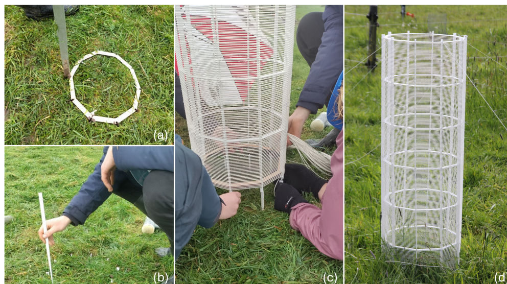
Figure 5. The coil installation process in the field. Firstly, an MDF template is used to pre-drill stake holes using a metal stake (a). Secondly, the individual stakes are pushed into the soil (b). The coil is then slotted into the tops of these stakes and fastened using the appropriate glue (c). The top of the coil is tethered to the soil by spanning 0.5 mm nylon fishing wire in four directions. Panel (d) depicts the coil installed in the field.
