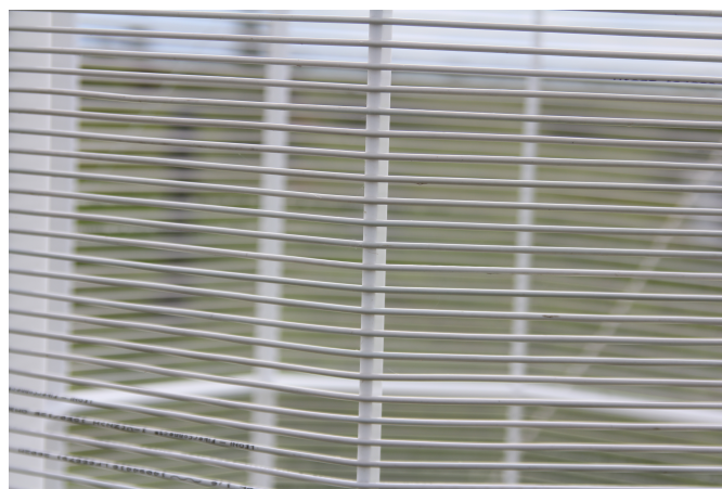
Figure 2. Close up of the coil. The fiber optic cable is kept firmly in place due to the notches on the ribs. Fiber position and spacing is accurately defined as can be seen in the image.
