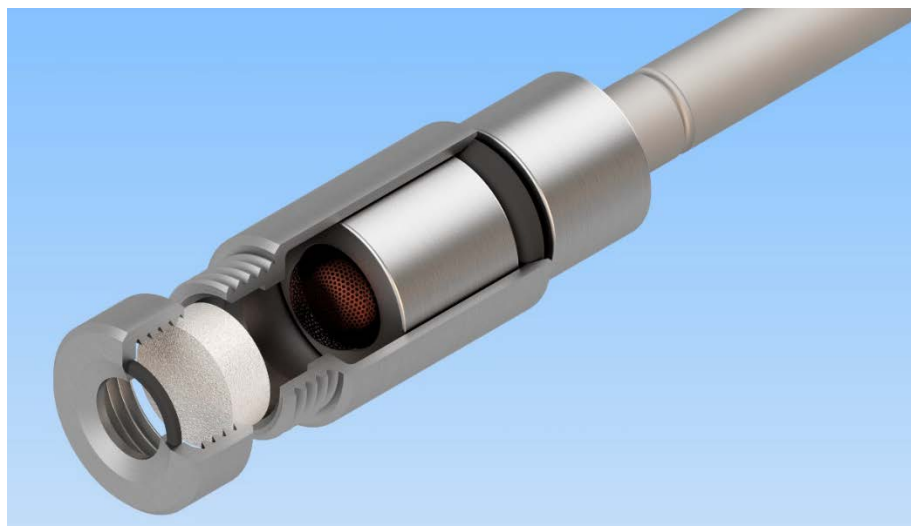
Figure 1. Schematic layout of the ozone scrubber. The scrubber housing was designed to fit on a commonly used diffusion-locking cap. Sample air flows from the left to the right, passing both a loaded glass filter as ozone scrubber and copper wool. A screw cap facilitates the quick and easy exchange of the filter. Two O-rings, located between the screw cap and the filter and between the housing and the diffusion-locking cap, prevent sampled air from bypassing the filter.
