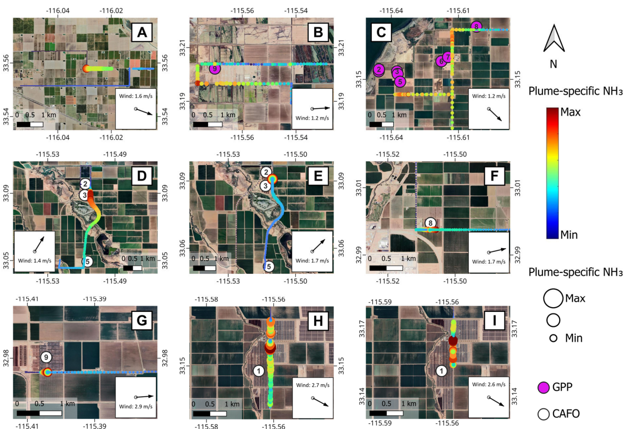
Figure 8. Time series of instantaneous ground-level \text{NH}_3 concentrations (ppb) measured by the mobile platform on each measurement day, with individual plumes labeled A to I for further investigation.
