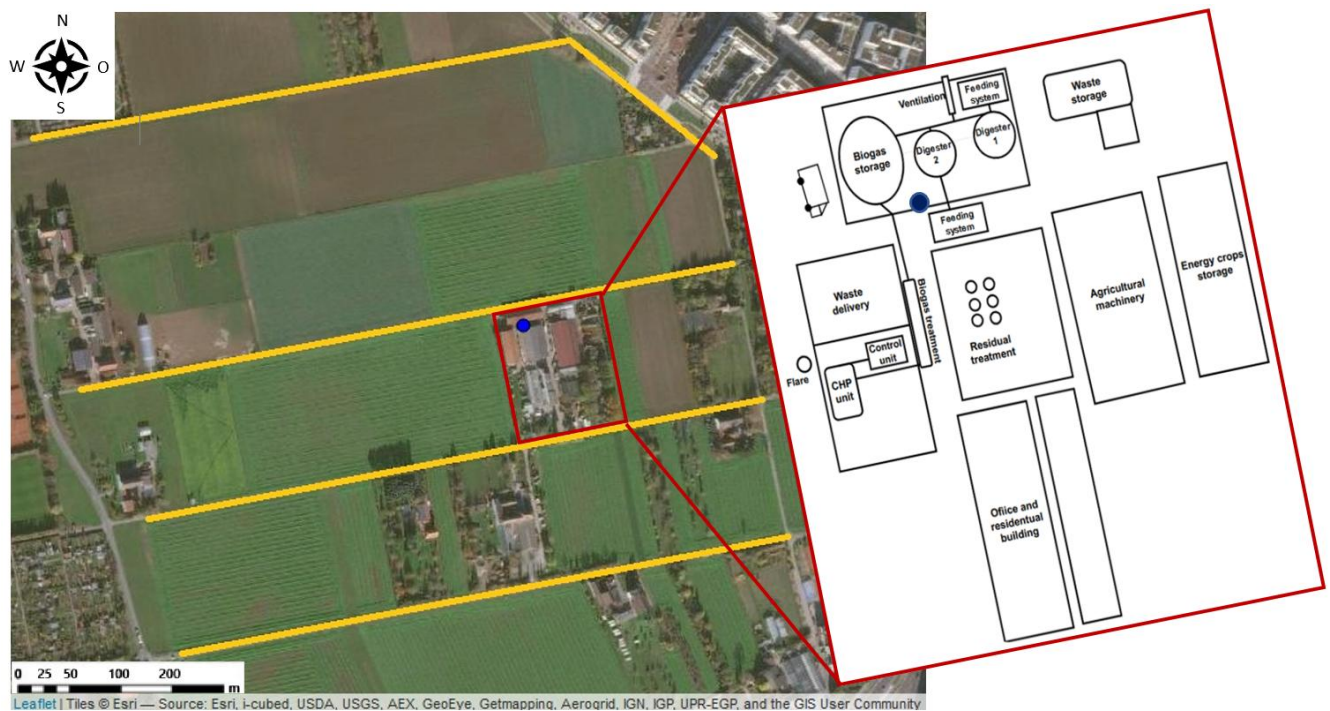
85 Figure 1. Map of the biogas plant site near Heidelberg, with the emission source location selected for implementing the GPM marked as a blue dot. A zoomed-in schematic of the plant shows the locations of the digesters, biogas storage, and CHP unit. Roads accessible for driving are marked in yellow. The map was created using Leaflet for R.
