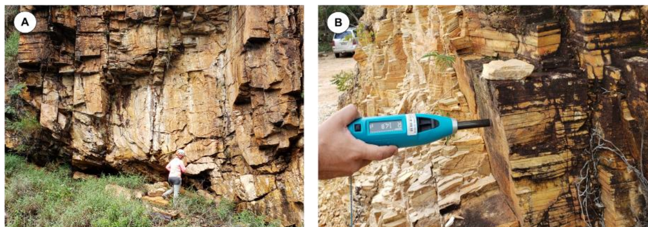
Figure 3: Field investigations. A) Structural data measurements. B) Schimdt Hammer sampling.
