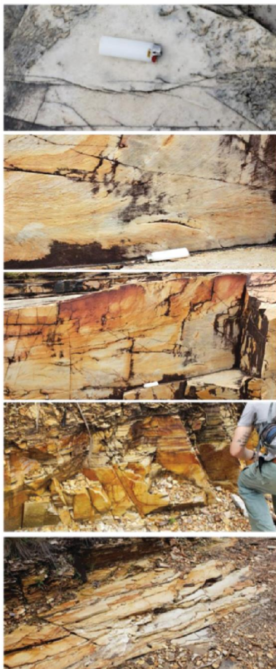
360 Figure 10: Different weathering degrees observed in the bedrock.
