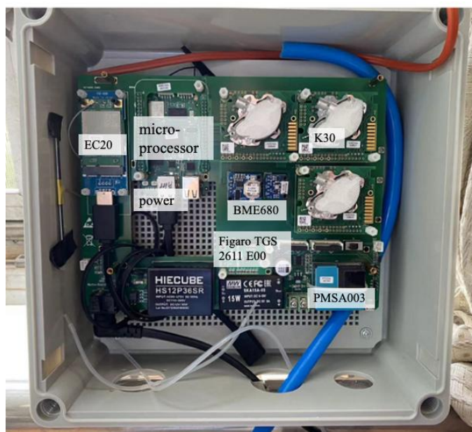
Figure 1. The layout of sensors in the standard version of SENSE-IAP instrument.
