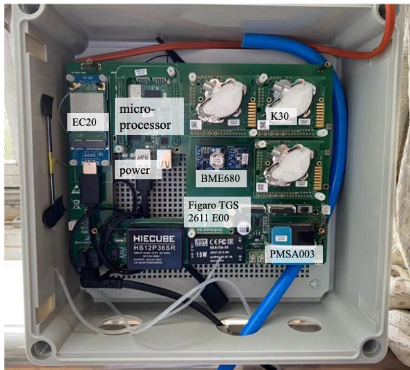
130 Figure 1. The layout of sensors in the standard version of SENSE-IAP instrument.
