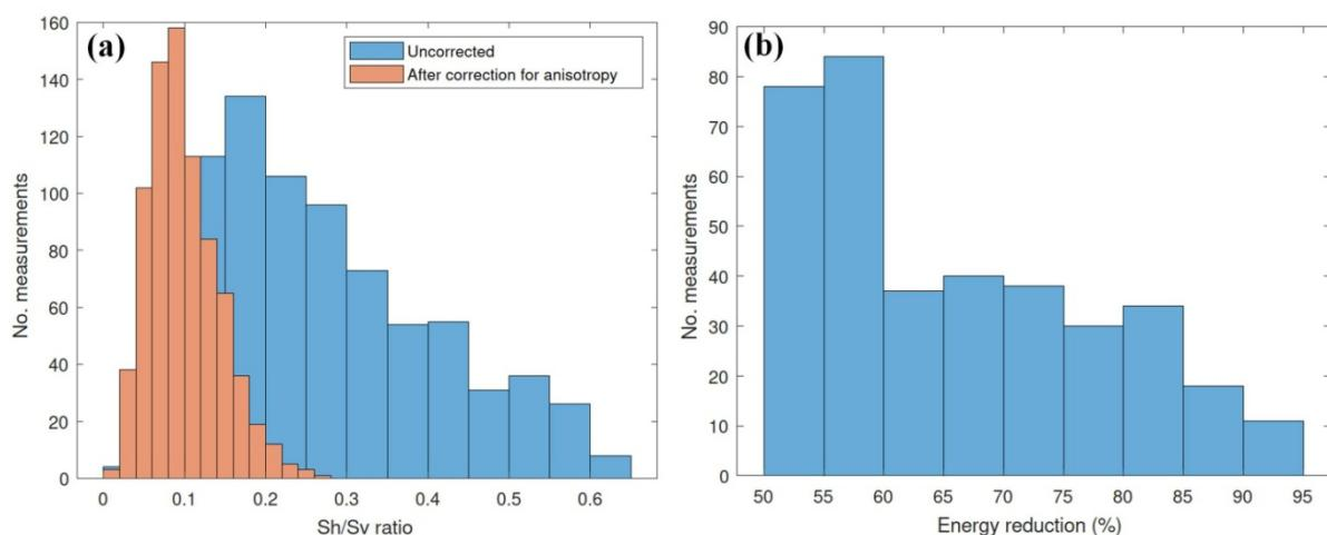
As shown in this Figure (panel b), reductions of T-component energy up to 95% are observed, but most measurements cluster between 50% and 60%. The T/R energy ratio is already low before correction (panel a, blue charts), so only moderate energy reduction is expected after
