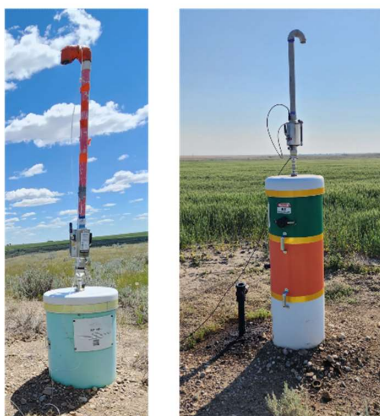
70 Figure 1: Overview of the test system used to emulate emissions in comparison to the configuration used to measure emissions in the field. (a) A conceptual diagram alongside (b) a mass flow meter (MFM) test system setup in the field. (c) a diagram of the deployment of MFM measurement systems quantifying orphan wells emissions and (d) photos showing measurement systems with different size chambers and vent pipe configurations. (Photo sources: Karl Haase (c) and Nicholas Gianoutsos (d), USGS).
