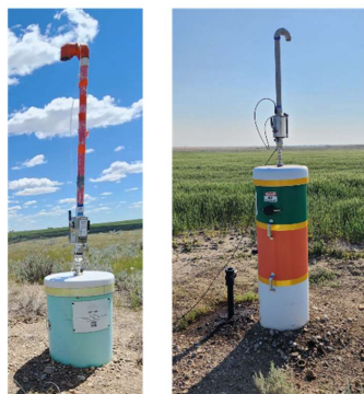
Figure 1: Overview of the test system used to emulate emissions in comparison to the configuration used to measure emissions in the field. (a) A conceptual diagram alongside (b) a mass flow meter (MFM) test system setup in the field. (c) a diagram of the deployment of MFM measurement systems quantifying orphan wells emissions and (d) photos showing measurement systems with different size chambers and vent pipe configurations. (Photo sources: Karl Haase (c) and Nicholas Gianoutsos (d), USGS).
