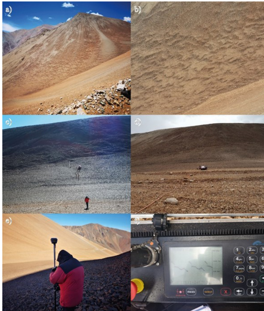
Figure 5. Photography of the fieldwork. (a) And (b) the Lobulated morphology of studied gelifluction taluses, which are not covered in snow; (c) and (d) the geoelectric line cable; (e) and (f) the used equipment, differential GPS and resistivity meter ARES II measuring a resistivity point diagram distribution.
