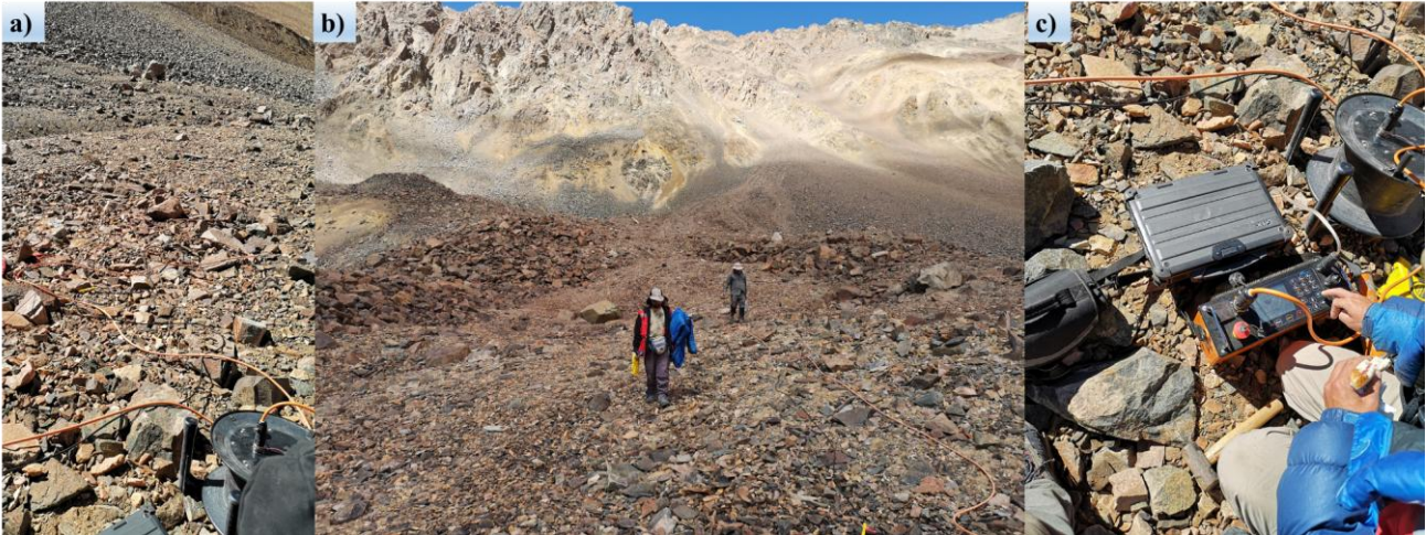
Figure 6. Photography of the fieldwork rock-glacier surface. (a) Intelligent multi-electrode cable reel used for deploying the ERT array across the periglacial terrain. (b) Installation of the 600-m geoelectric line. (c) Operation of the ARES II resistivity meter during data acquisition.
