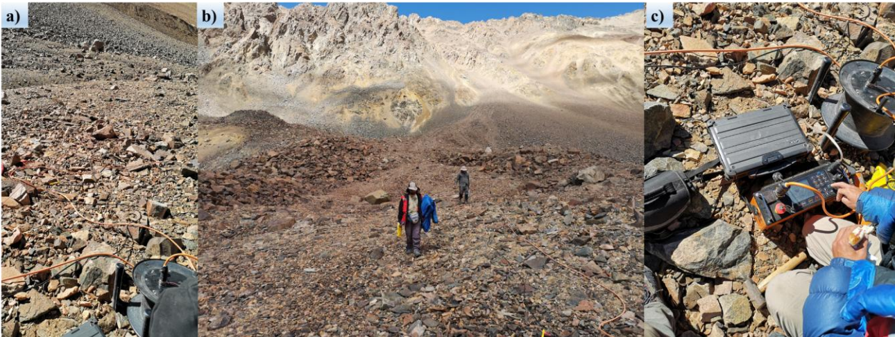
Figure 6. Photography of the fieldwork rock-glacier surface. (a) Intelligent multi-electrode cable reel used for deploying the ERT array across the periglacial terrain. (b) Installation of the 600-m geoelectric line. (c) Operation of the ARES II resistivity meter during data acquisition.
