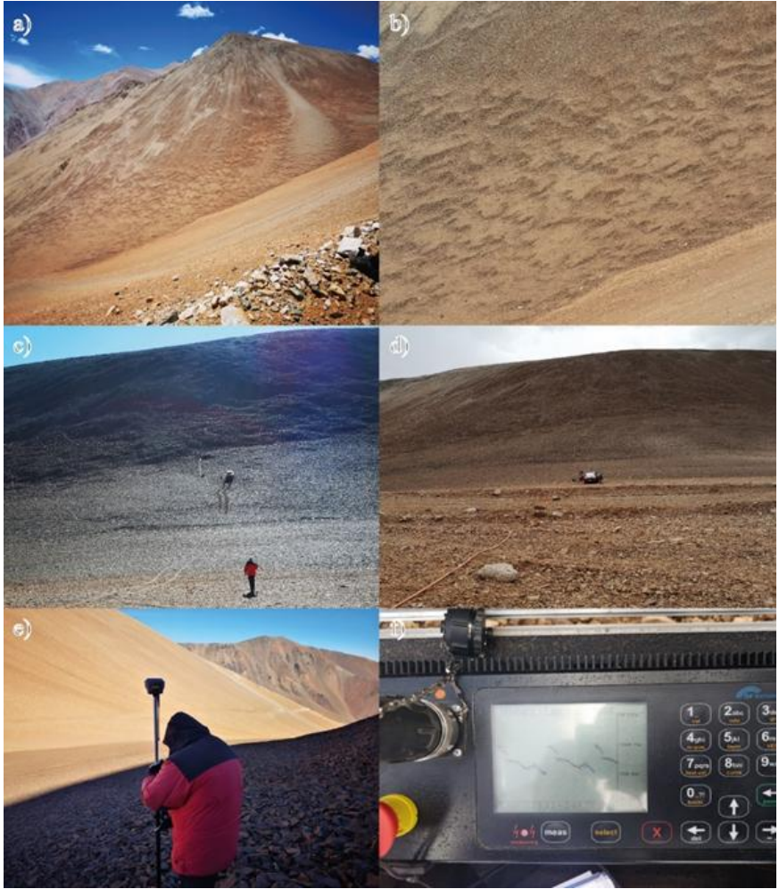
322 323 Figure 5. Photography of the fieldwork. a) And b) the Lobulated morphology of studied gelifluction taluses, which are not covered 324 in snow; c) and d) the geoelectric line cable; e) and f) the used equipment, differential GPS and resistivity meter ARES II measuring 325 a resistivity point diagram distribution.
