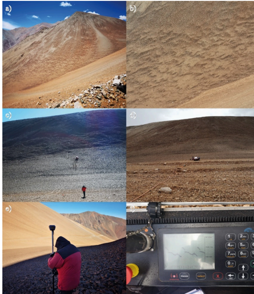
Figure 3. Photography of the fieldwork. a) And b) the Lobulated morphology of studied gelifluction taluses, which are not covered in snow; c) and d) the geoelectric line cable; e) and f) the used equipment, differential GPS and resistivity meter ARES II measuring a resistivity point diagram distribution.
