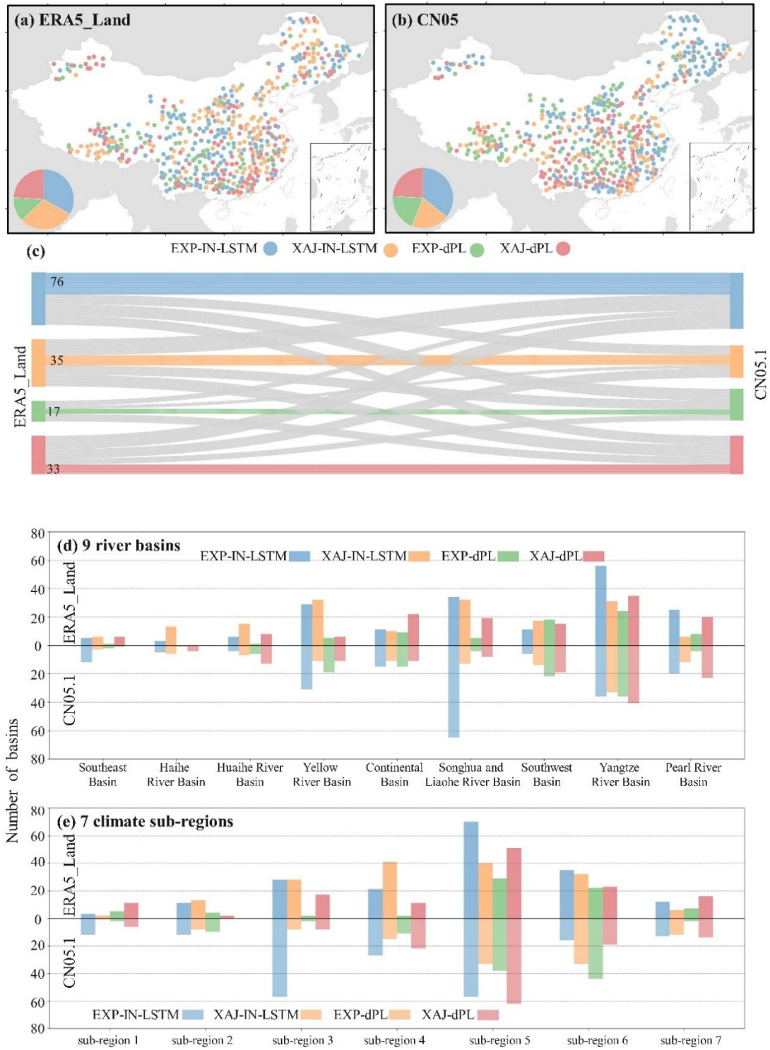
Figure 11. Comparison of hybrid model performances across basins using ERA5-Land and CN05.1 precipitation data. (a) Spatial distribution of the best-performing hybrid models under ERA5-Land forcing. (b) Spatial distribution under CN05.1 forcing. (c) Sankey diagram showing the consistency of best-performing models across datasets. (d) Number of best-performing basins for each model in the 9 major river basins. (e) Number of best-performing basins in the 7 climate sub-regions.
