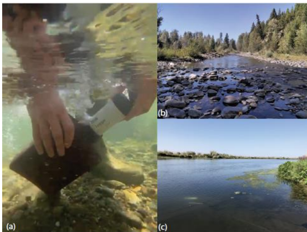
Figure 1. Modified semi-in situ dark bottle incubation method and example study sites. (a) Underwater photograph of DO sensor being inserted into an incubation bottle filled with river water and mixing device. Right panels emphasize the diversity of environmental settings covered in this study. (b) North Fork Teanaway River (site S19E), Kittitas County, Washington, September 2021. Site S19E is classified as a mesic, high elevation site dominated by tree canopy (Cluster 1; see Table 1, Table S3, Fig. S1). (c) Yakima River at Mabton (site T02), Yakima County, Washington, September 2021. Site T02 is classified as a mesic, middle elevation site dominated by tree canopy (Cluster 5; see Table 1, Table S3, Fig. S1).
