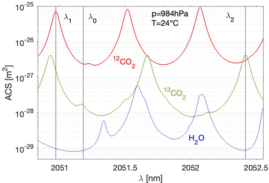
Figure 1: Absorption cross-section (ACS) for <sup>12</sup>CO<sub>2</sub>, <sup>13</sup>CO<sub>2</sub> and H<sub>2</sub>O for pressure 984 hPa and temperature 24°C (Voigt profile). Isotopic ratio is taken into account. The DIAL wavelengths chosen in this work are indicated.
