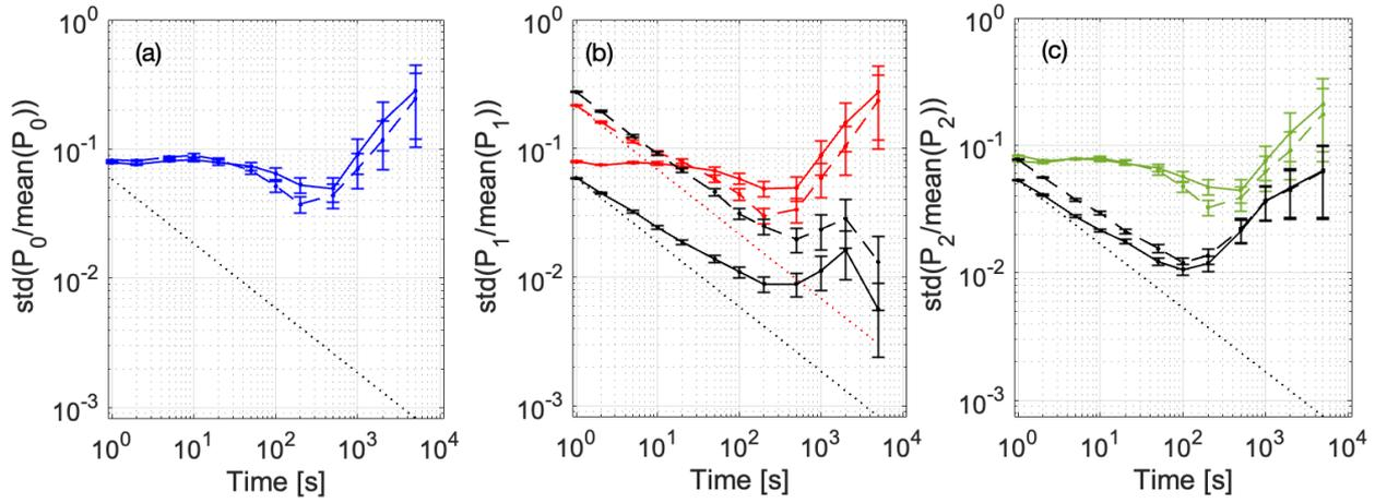
**Figure 4: Allan deviation at R=0.5 km (solid line) and R=1.5 km (dashed line) for (a)  $\lambda_0$  (b)  $\lambda_1$  (red) and  $P_1/P_0$  ratio (black), (c)  $\lambda_2$  (green) and  $P_2/P_0$  ratio (black). The dotted lines are indicated for the standard white noise deviation ( $1/\sqrt{Time}$ )**
