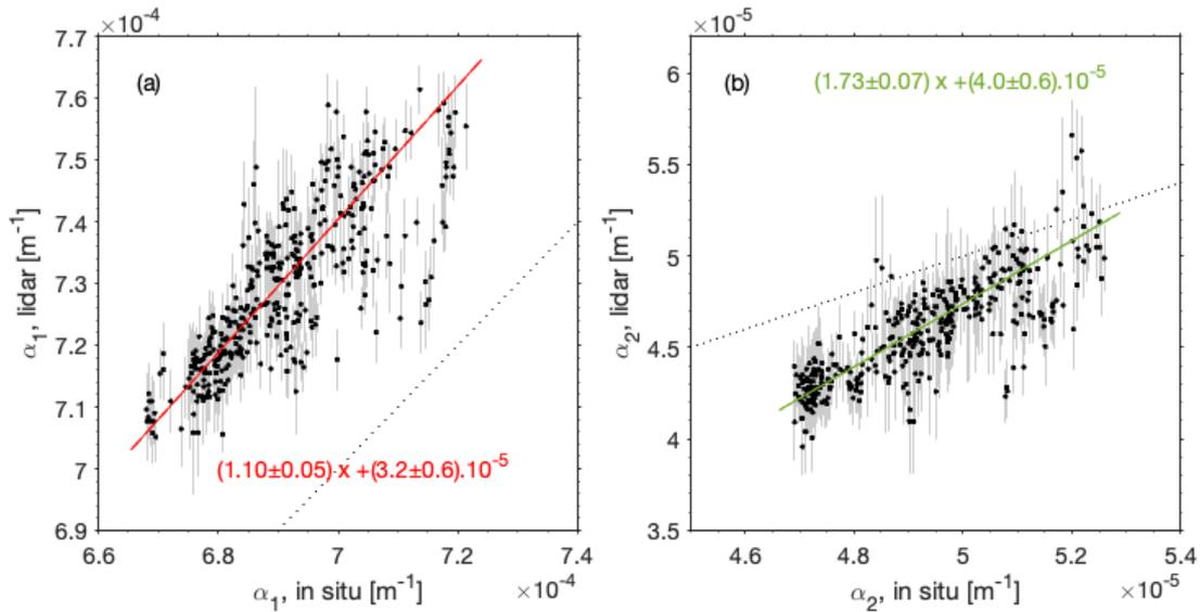
330 **Figure 7: Comparison between lidar and in situ differential absorption coefficient (from meteorological, spectroscopic and gas analyzer data) for wavelength 1 (<sup>12</sup>CO<sub>2</sub>) (a) and 2 (<sup>13</sup>CO<sub>2</sub>) (b). The dotted line is for  $\alpha_{i, \text{lidar}} = \alpha_{i, \text{in situ}}$ .**
