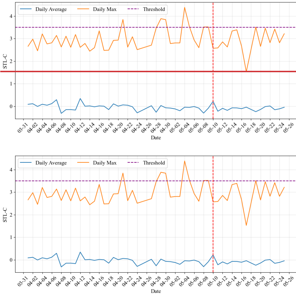
Figure 9: Variation Characteristics of STL-C Maximum and Average Values from April 1 to May 26, 2023. (Red Dashed Line Indicates the Time of Earthquake Occurrence)
