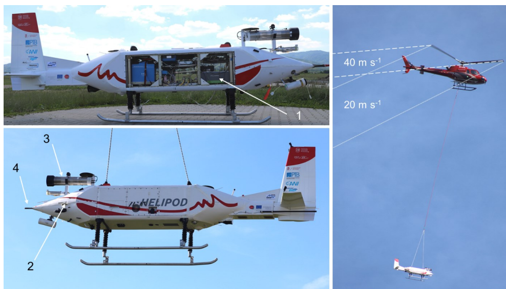
Figure 2. The helicopter-borne measurement system HELiPOD with instruments mounted inside and outside: Picarro G2401-m (1) with its inlet (2) for precise \text{CH}_4 measurements, Licor LI-7700 (3) for high resolution \text{CH}_4 measurements and a five-hole probe (4) for precise 175 wind measurements. The right picture illustrates the rotor downwash area for the air speed of 20 \text{ m s}^{-1} and 40 \text{ m s}^{-1} (adapted from Pätzold et al., 2023).
