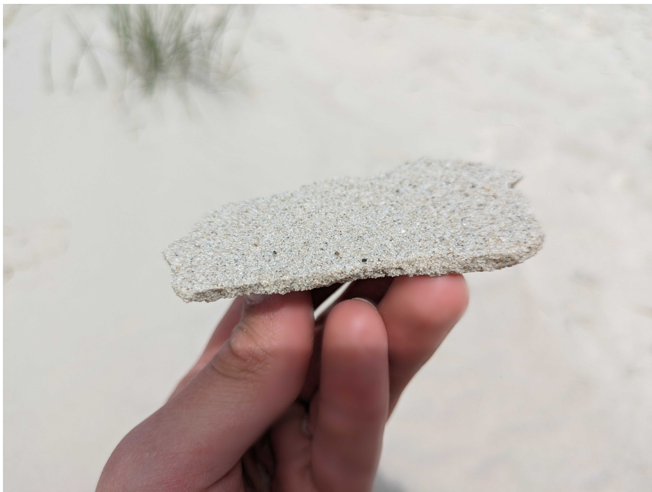
Figure A6. Stable piece of the crust which could be lifted and did not fall apart on its own
