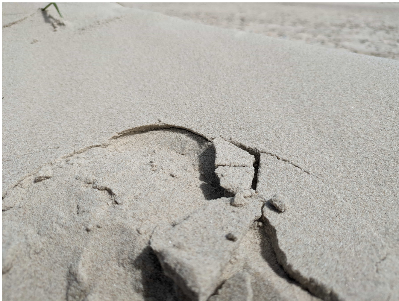
Figure A4. The crust formed a continuous layer with dry powder sand beneath
