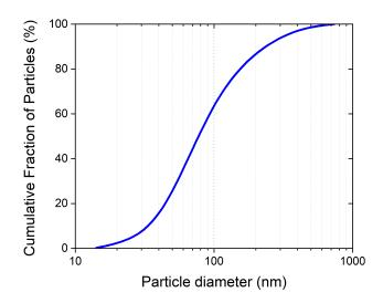
Cumulative size distribution (percentual) of the silica particles used in the IN experiments.
