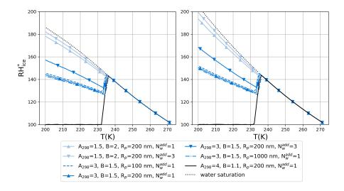
Comparison of critical relative humidity with respect to ice  $(RH_{ice}^*)$  as a function of temperature (T) for different parameter sets.
