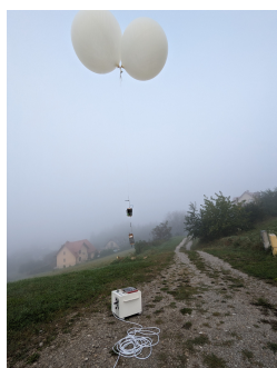
(a) Balloon with attached payload and connected to the winch.
