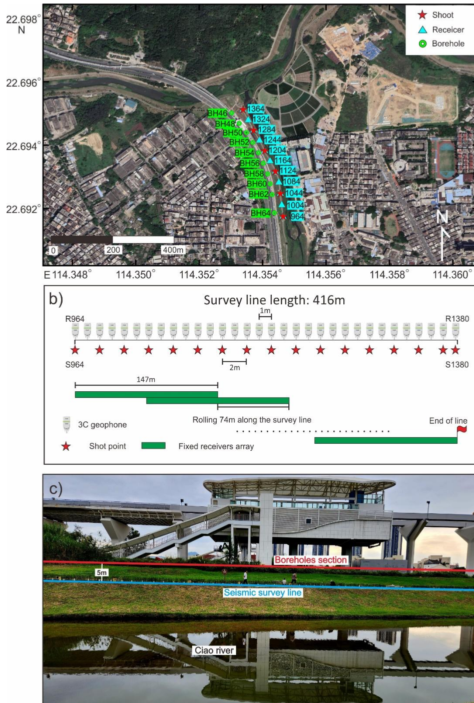
Figure 3: (a) Locations of receivers (cyan triangles), shots (red stars) and boreholes (green dots), (b) Geometry of the seismic acquisition profile, receiver spacing 1 m, shot spacing 2 m, separated into five segments, each segment consisted of 148 fixed units with 74 units overlapping, (c) Field work photo of the seismic survey line (cyan line) and geological section consisting of 19 boreholes (red line), the geological section is 5 m higher than the seismic survey line (the aerial image from Google Maps).
