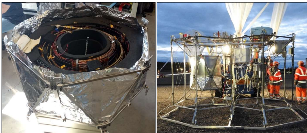
Figure 1: Left: The MegaAirCore (MAC) tubing inside its two layers of insulation. Also visible are several of the temperature sensors deployed to monitor the temperature of the tubing in various places. Right: Gondola just before launch with the MAC parcel mounted low inside the lefthand side hexagon, and the cryosampler inside the righthand side one. Copyright J. C. Laube (left) and CNES/Prodigima - R. Gaboriaud (right).
