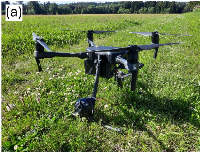
10 Figure S1: Photo of the filter holder attached to the landing gear at the drone dji m300 (a) and at plate between the landing gear of the dji m200 (b).
