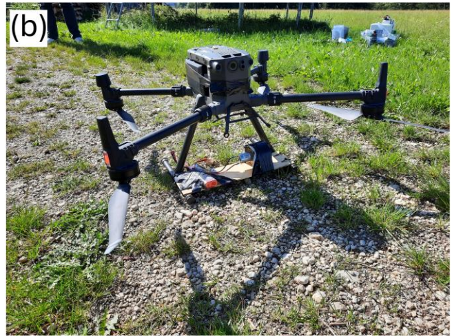
10 Figure S1: Photo of the filter holder attached to the landing gear at the drone dji m300 (a) and at plate between the landing gear of the dji m200 (b).
